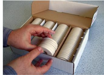
2. Position the Bullers Rings onto the kiln in accordance with a predetermined plan. Mark the position numbers onto the Bullers Rings for the purpose of mapping the kiln firing, and detail this onto the kiln record sheet.
