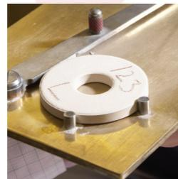
In the case of the Vector Gauge, insert the ring between the two converging guide rails and the reading from the top of the disc against the engraved scale.
