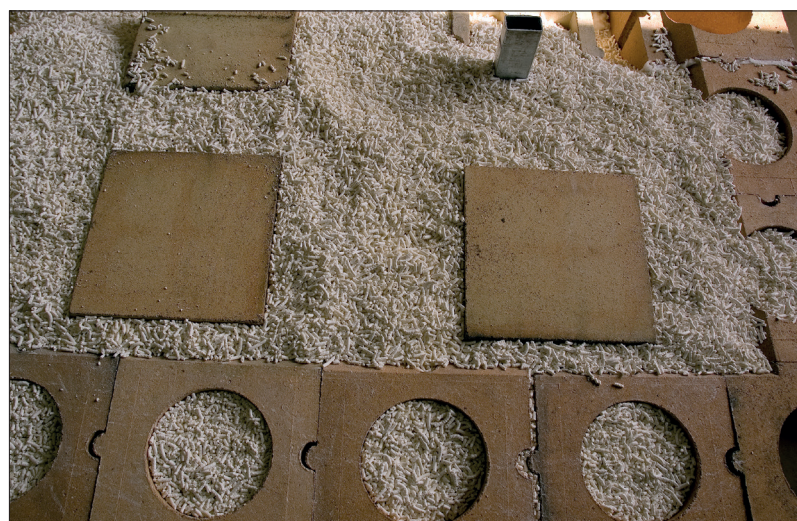
Fig. 5 Ultralite – highly effective insulation in kiln cars
