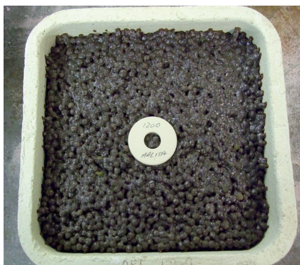
Fig. 3 Expanded clay aggregate under firing trial at 1200 °C
