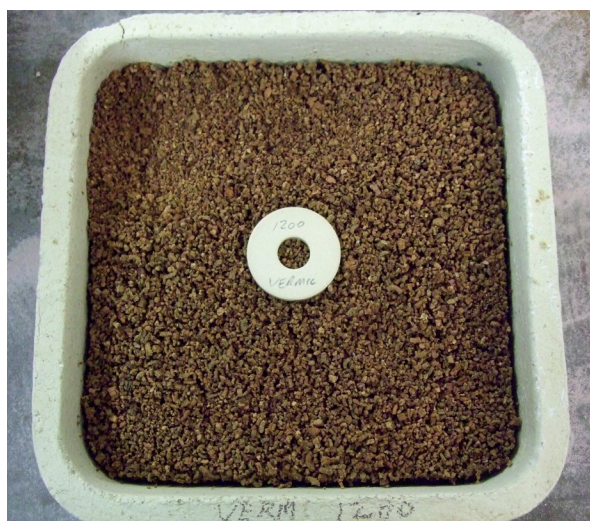
Fig. 1 Vermiculite under firing trial at 1200 °C
