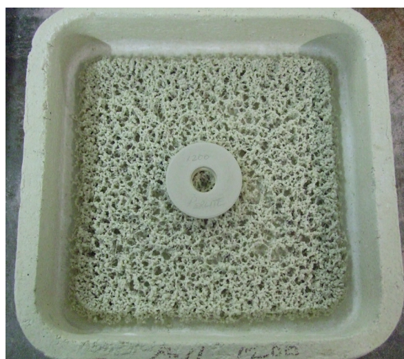
Fig. 2 Perlite under firing trial at 1200 °C
