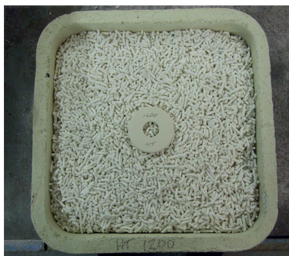
Fig. 4 Ultralite ULF-12 under firing trial at 1200°C
