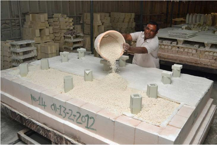
An efficient, low density insulation material was the target to help reduce the amount of energy consumption within the kiln car base. Anchor decided to completely redesign the kiln car to maximise the Ultralite benefit, this included new lightweight periphery blocks, new kiln furniture and supports all of which contributed to the saving. Clearly, in volumes terms the construction was made up largely of Ultralite to a depth of 340mm, topped with a 12mm fibre blanket.
