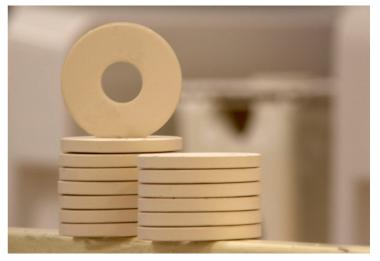
Bullers Rings provide an independent, accurate, reliable and essential indication that the firing of the product is correct and unaffected by any variations in temperature and kiln loading.
