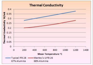
The density, heat stored and heat loss data has been calculated based on a 240mm thickness at a hot face temperature of 1400°C (2552°F) using SIMUTHERM Heat Flow Simulation Software.
